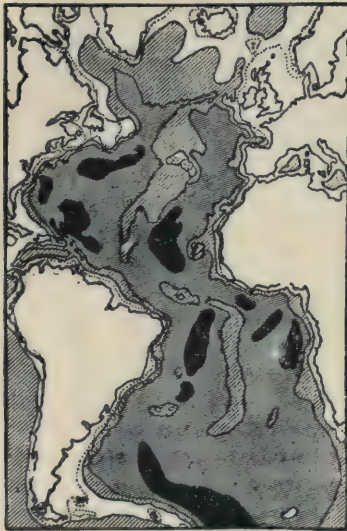
FIG. 37.—Configuration of the Bed of the Atlantic Ocean, showing contour lines of 100 fathoms (dotted), 1,000, 2,000 and 3,000 fathoms of depth. All over 3,000 fathoms is in solid black.
